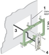
Using the supplied mud ring as a guide, mark and cut out the appropriate material within the marked area.
