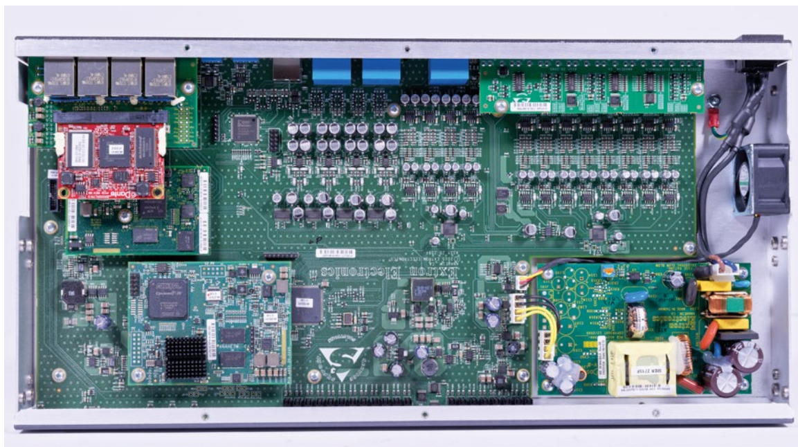
Image 06: The DMP 128 Plus is built with a large base board and various plug-on modules. The separate power supply unit is on the bottom right.
