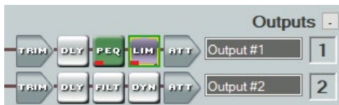
FIG. 05: Modules for signal processing in the analog output channels and expansion outputs
