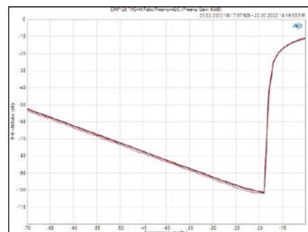
Fig. 09: THD+N depending on the input level (x-axis) at 0 dB gain (top) and 40 dB gain (bottom). Measurements at 100 Hz(- - -), 1 kHz( ) and 6.3 kHz(...).
