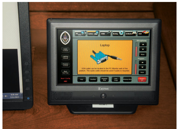
A TLP Pro 720T touchpanel provides intuitive control of AV system operation.
