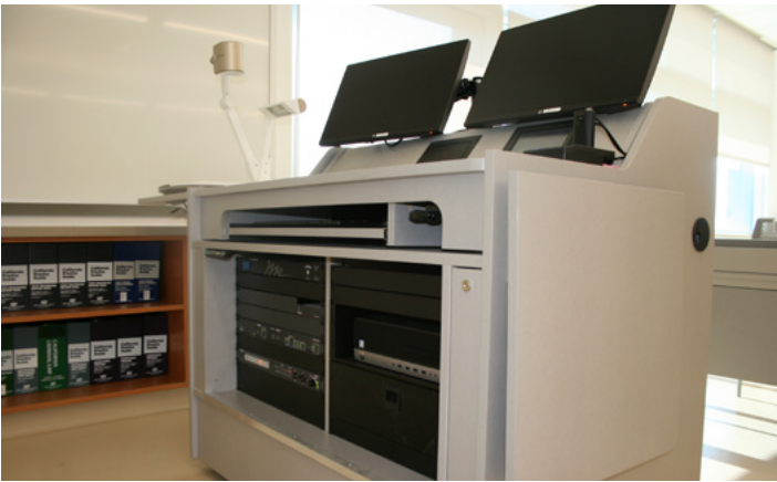
AV system components had to fit within the ADA-compliant teaching station that Marshall Furniture custom designed for Mt. San Antonio College.
