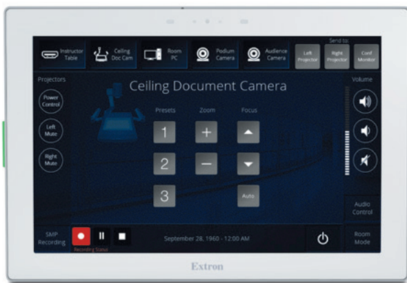
AV system functions in the training classrooms are controlled via TouchLink Pro touchpanels.
