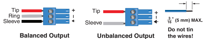
Figure 4. Output Wiring
